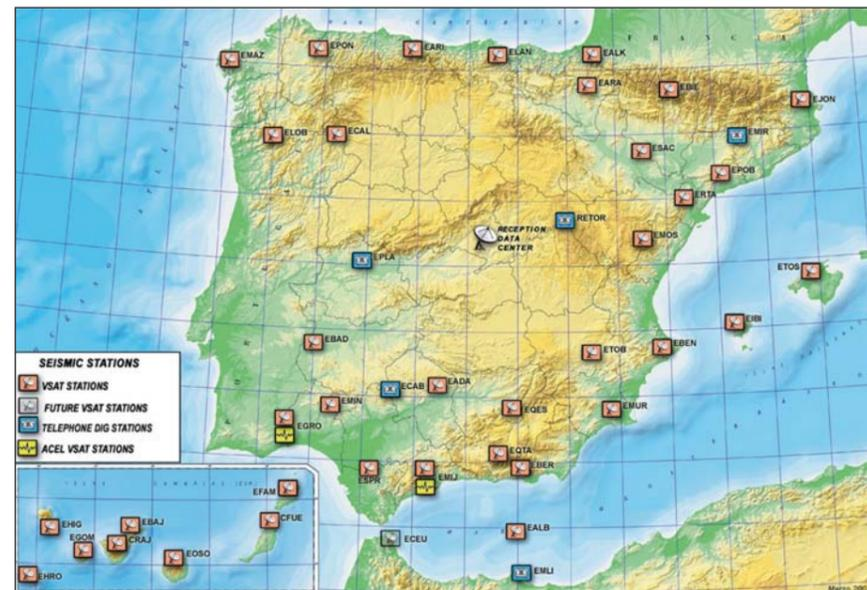
Since 2000 February, the IGN has developed its new Seismic Network. Nowadays, 29 stations are placed in the peninsular area and other eight in Canary Islands, one per island except two in Tenerife Island. All of them are digital broad band stations, with three components and VSAT telemetry. IGN is planning to install some additional stations in the future. In the following weeks a new VSAT station will be installed in North Africa (Ceuta).
