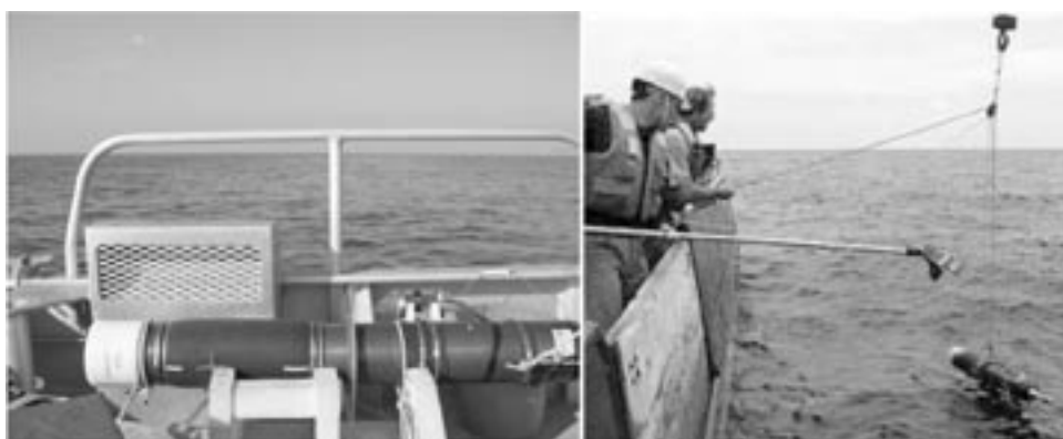
Figure 1. The first MERMAID prototype, equipped with a hydrophone (left) being launched for testing (right). Figure courtesy of Frederik Simons.
