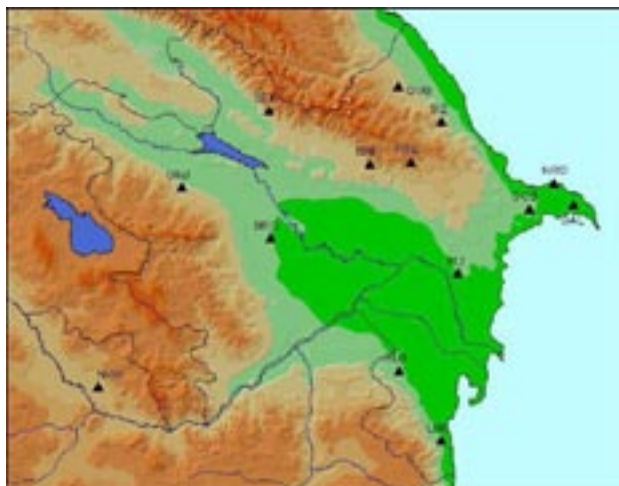
Figure 2: Map of allocation of the new digital seismological network in Azerbaijan.
