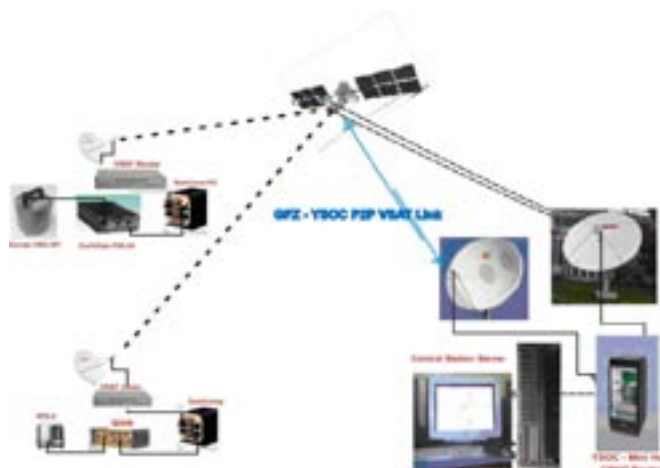
Fig.3: The diagram shows the layout of the new seismic monitoring system using VSAT communication.
