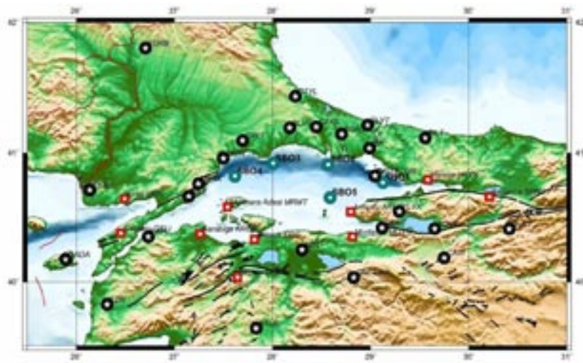
Fig.3: Locations of Sea Bottom Observatories (SBO) and distribution of Broadband Seismic Stations (BB) around the Marmara Sea area. (Blue symbols show SBO, red symbols show BB stations provided by Turkish Telecom, black symbols show existing BB stations)
