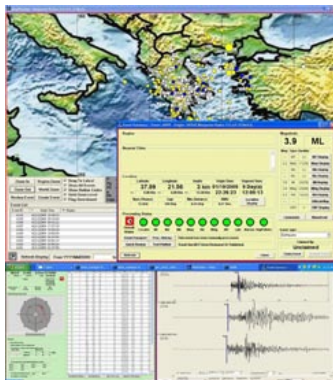
Figure 4: Example of Hydra system display. Location and phase picking windows are shown.
