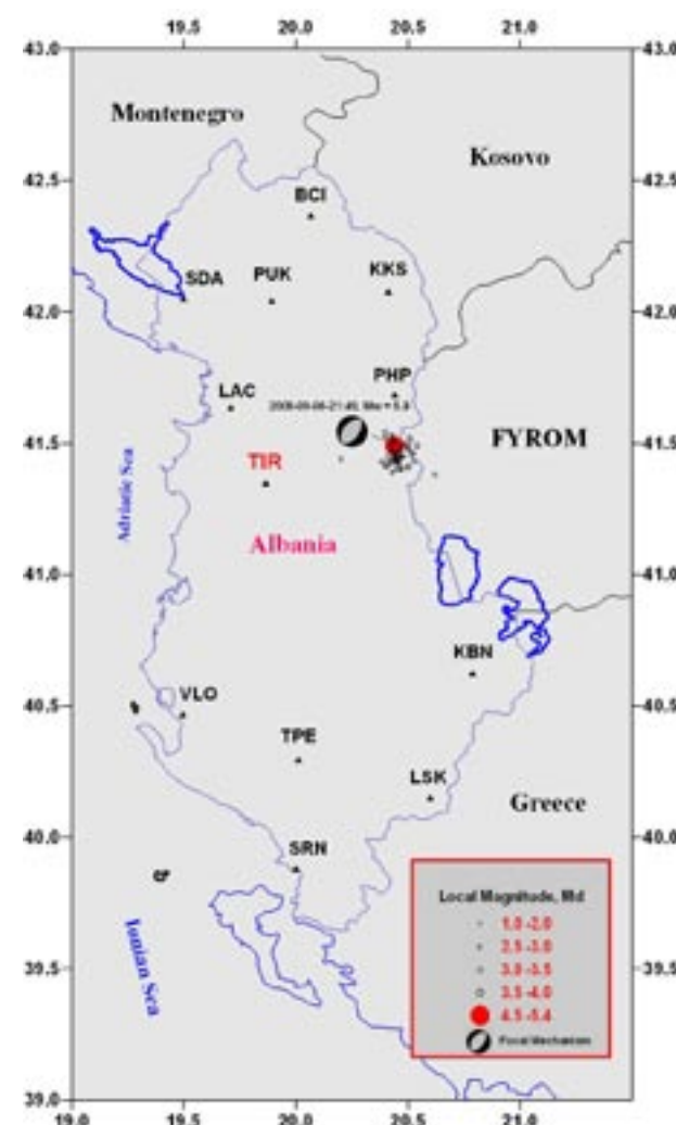
Figure 2 - Map of Areal distribution of seismic activity from September 6, and on; Main shock 2009-09-06-21:49 and subsequent aftershocks; Focal Mechanism solution; Seismological Stations of Albanian Seismological network.
