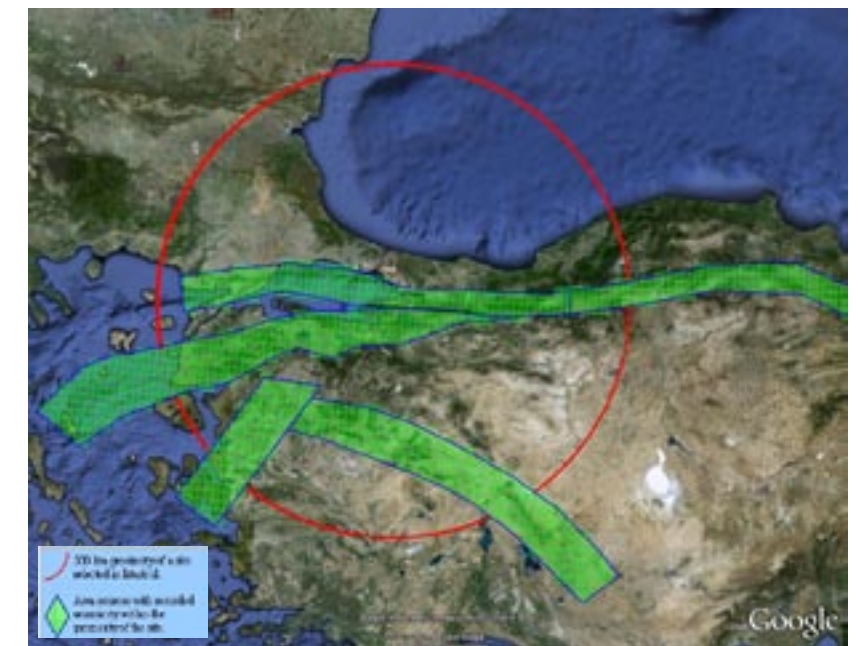
Figure 2 - An example of area sources used to generate the risk map of Istanbul by the SRA application
