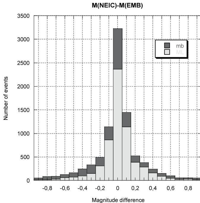
Figure 7: Comparison of mb and ML magnitudes computed at the NEIC and in the Euro-Med bulletin for all associated events. Mean values are  $-0.06$  for mb and  $0.02$  for ML. Associated standard deviations are  $0.49$  for mb and  $0.27$  for ML.
