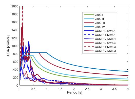
Figure 6. Comparison of the response spectra of Siahoo station with the spectra of national 2800 standard.
