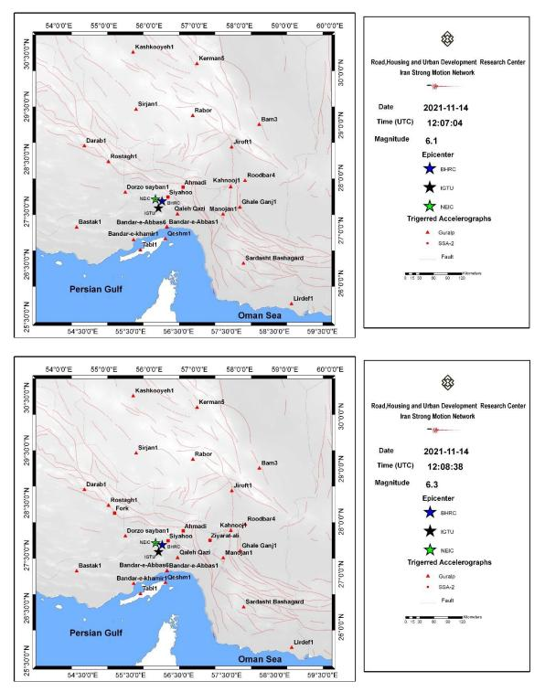
Figure 2 Map of the ISMN recording stations for the first (up) and the second (bottom) earthquake along with the epicenters reported by different agencies.
