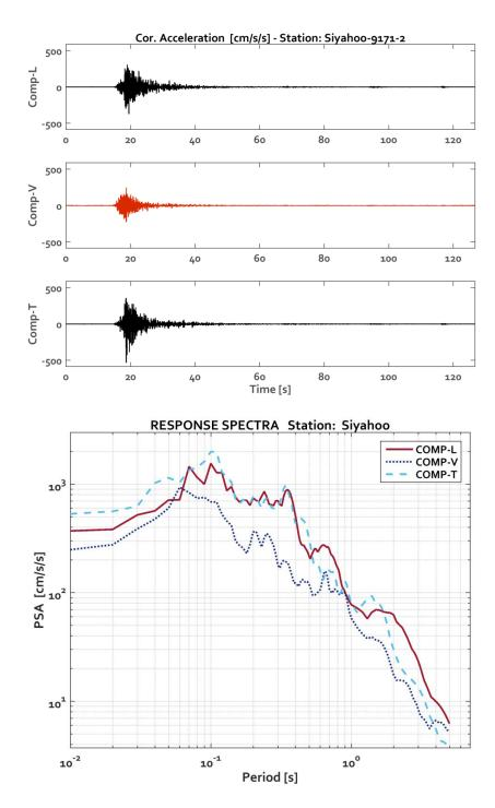
Figure 5. Recorded acceleration time histories (top) and acceleration response spectra of second earthquake at about 15 km epicentral distance.
