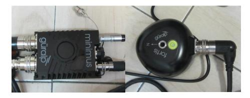
Figure 1. Fortis-Minimus accelerometers used in ISMN stations.
