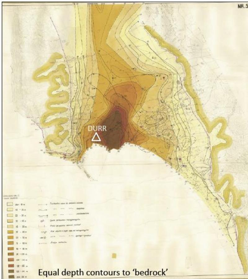
**Figure 4.** Equal depth to 'bedrock' contours map for the city of Durres according the microzonation project of Durres (Kociu et al., 1985).
