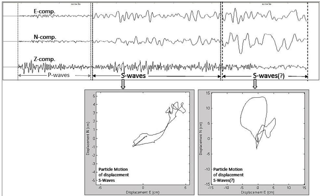
**Figure 11.** Displacement particle motion at the DURR station estimated for the first S-wave window and the second stronger part of S-wave(?) window of the mainshock.
