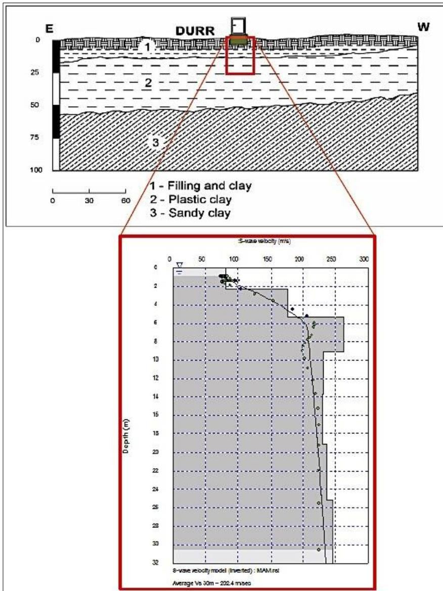
**Figure 6.** East-west cross section and lithology (upper) of the Durres basin (Koci, 2013); Vs profile of the DURR station for the upper 30m (lower) (Duni, 2013).
