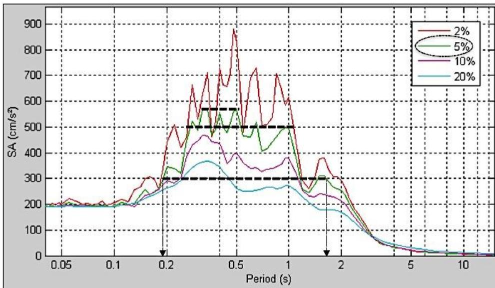
**Figure 8.** Pseudo-acceleration response spectra ( $D=0.02, 0.05, 0.1, 0.2$ ) of the first 15sec of the acceleration time history recorded at the DURR station.
