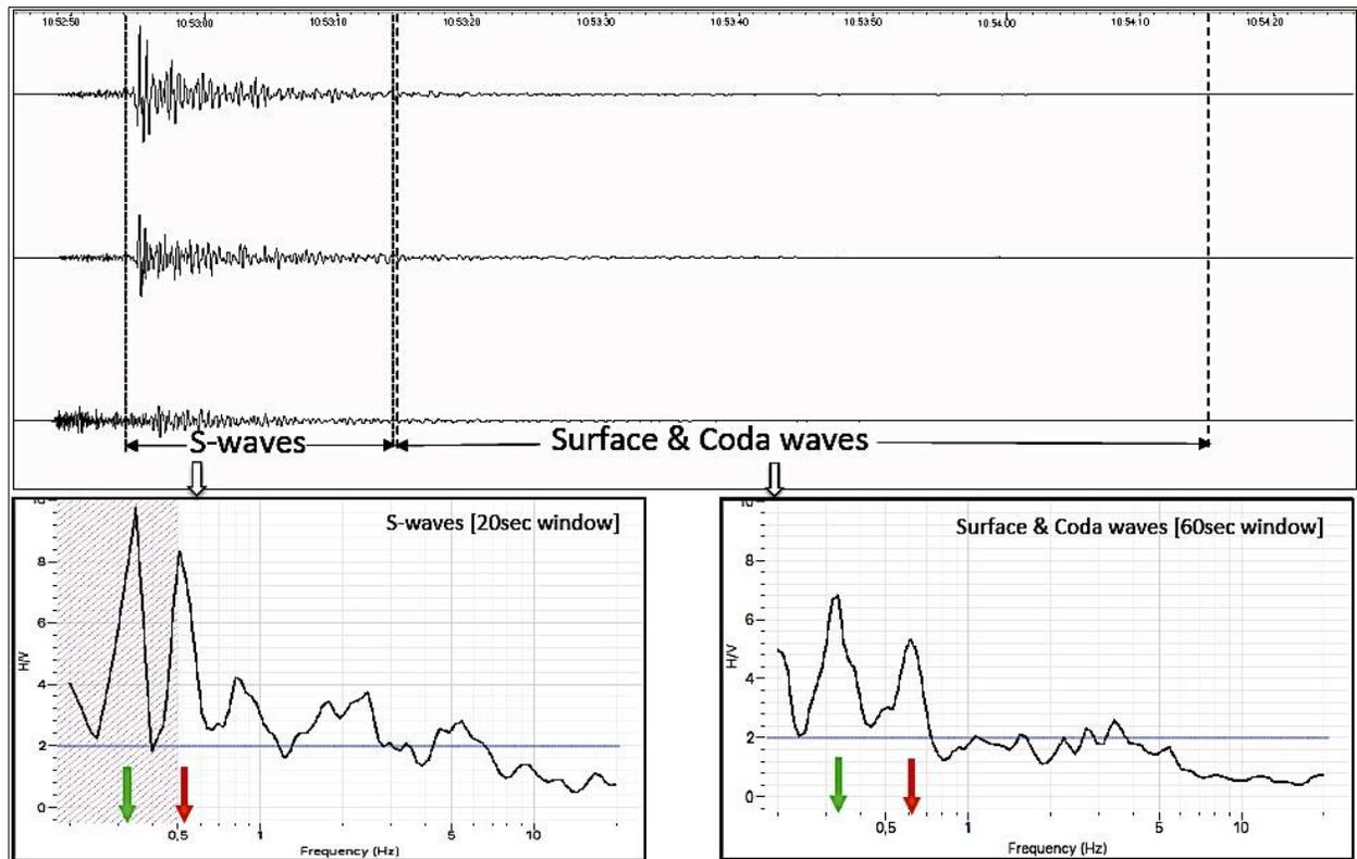
**Figure 14.** Horizontal-to-Vertical Spectral Ratio (HVSr, Receiver Function) at the DURR station estimated for the S-wave window and the surface & coda waves window of the aftershock of 28/11/2019, 10:52:44 (M4.6).
