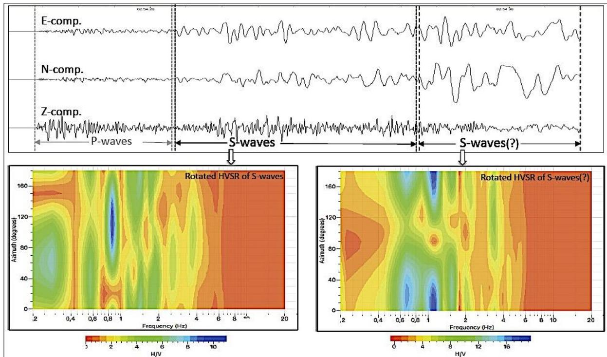
**Figure 12.** Horizontal-to-Vertical Spectral Ratio (HVSr, Receiver Function) at the DURR station estimated for the first S-wave window and the second stronger part of S-wave(?) window of the mainshock.
