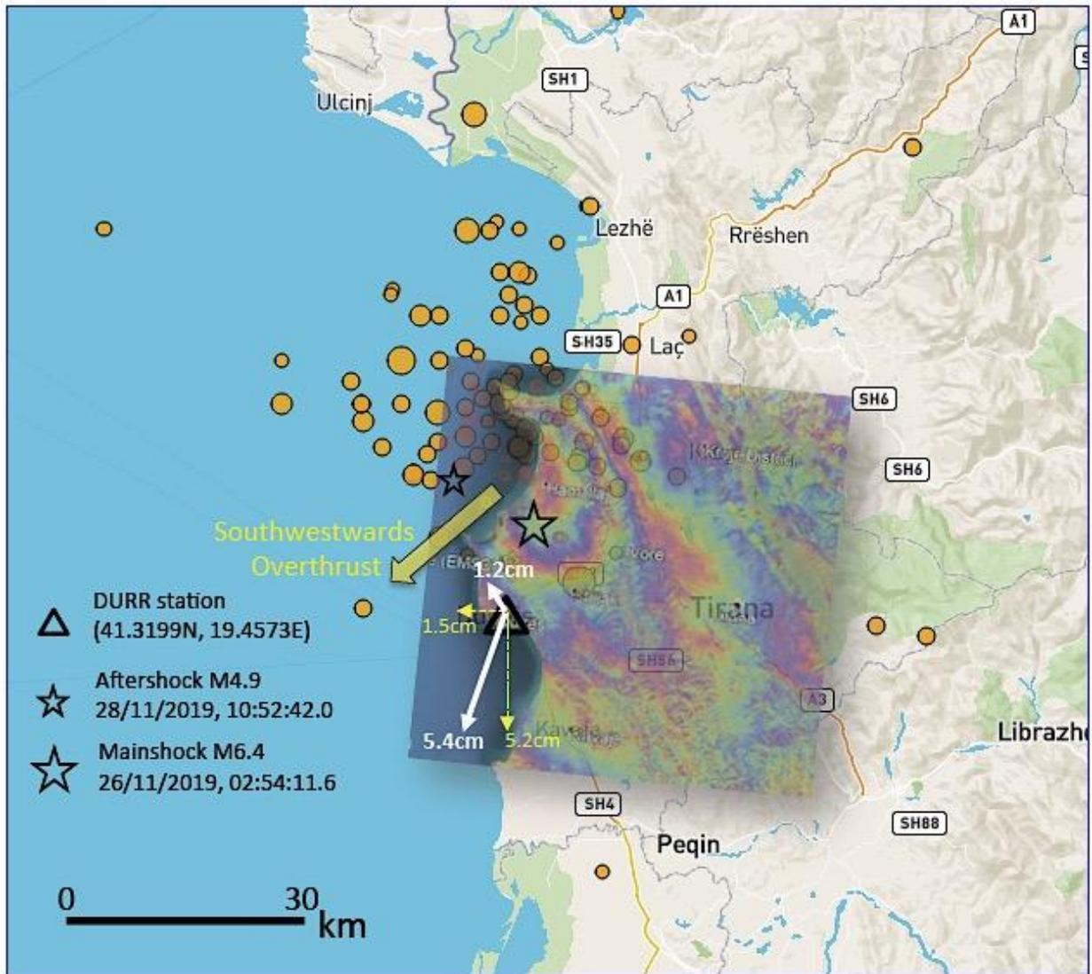
**Figure 10.** Horizontal and vertical permanent displacements (white arrows) estimated from the acceleration time history of Durrës (DURR station); two weeks aftershock activity (AUPh Seismological Station & EMSC); interferogram for the mainshock (Tsironi and Ganas 2019).
