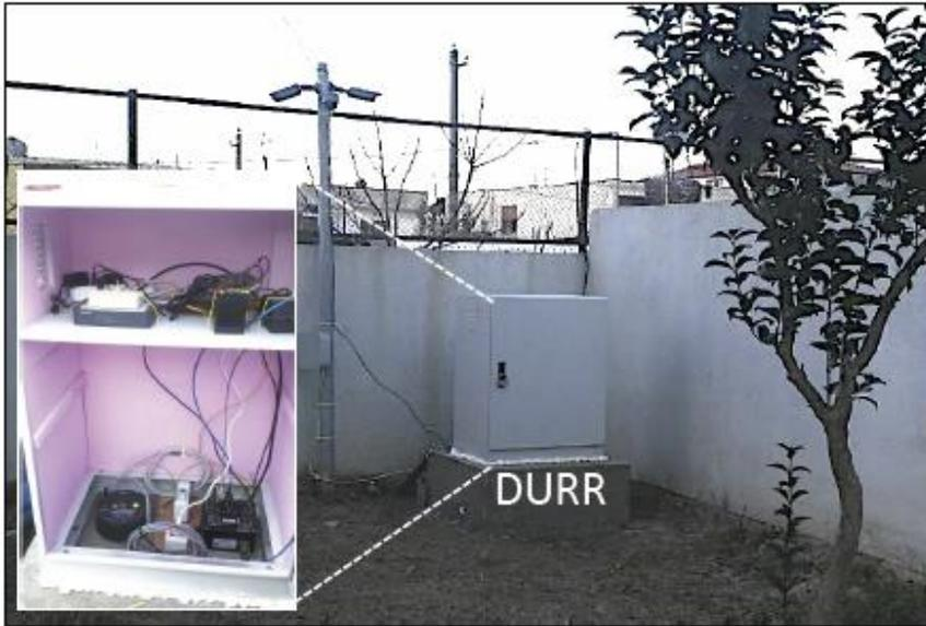
**Figure 5.** Durr free-field accelerometric station (CMG-DM24).
