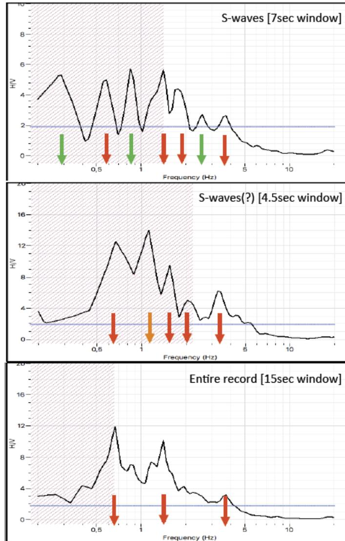
**Figure 13.** Horizontal-to-Vertical Spectral Ratio (HVSR, Receiver Function) at the DURR station estimated for the first S-wave window(upper), the second S-wave(?) window (middle) and the entire record length of the mainshock (down).
