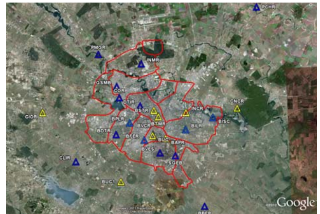
Bucharest seismic network: yellow triangles represent real-time stations and blue triangles represent offline stations
